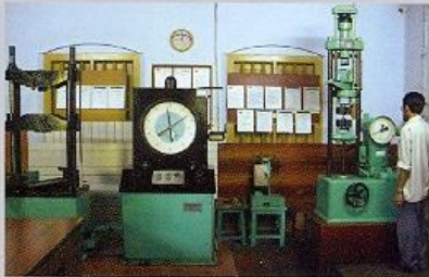
Mechanical Testing for M.O.R., Compression, Tensile, Shear and Impact
